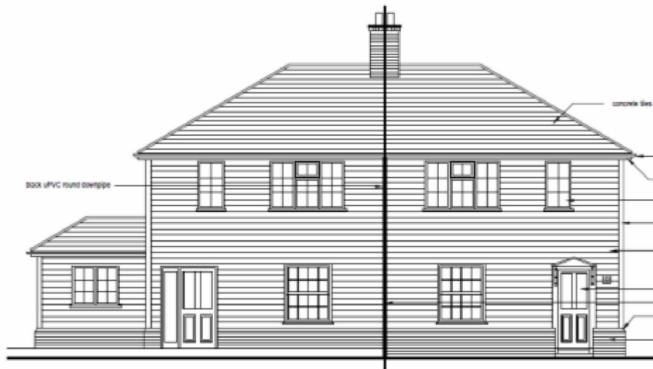
Fig. 16: New flush casement and sliding sash metal windows will enhance the fenestration. The two, ground floor, front elevation windows will both be sliding sashes, as per the original design intent.
